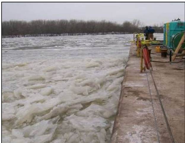
Figure 4 – Ice Accumulating at Lead Edge of Barge
