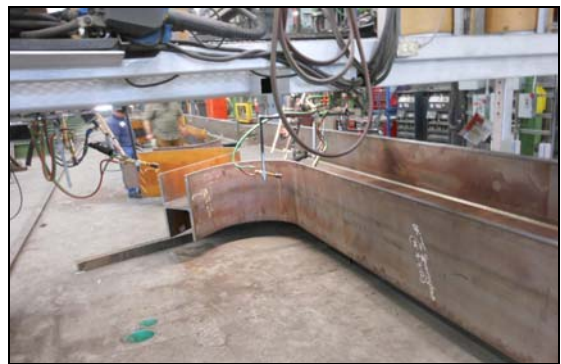
Figure 16 – Cold-formed steel truss chords shown during fabrication
