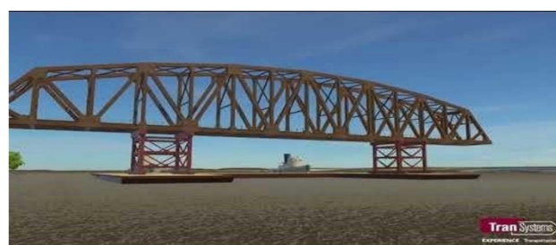
Figure 1 - Float-in Concept Developed by EOR
