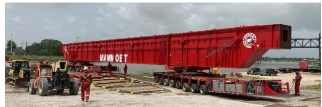
Figure 14 - PDV beam being loaded onto deck barge
