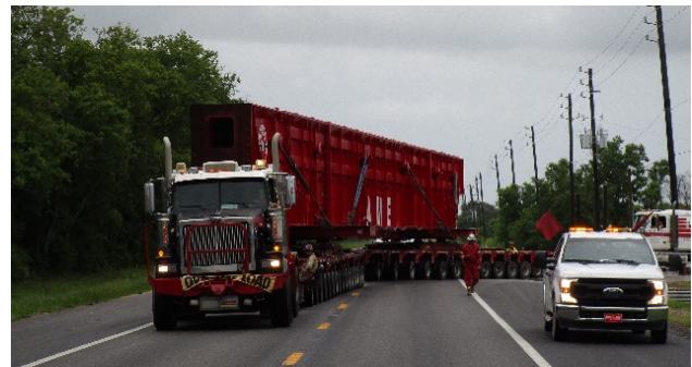
Figure 13 - PDV beams transported using SMPTs
